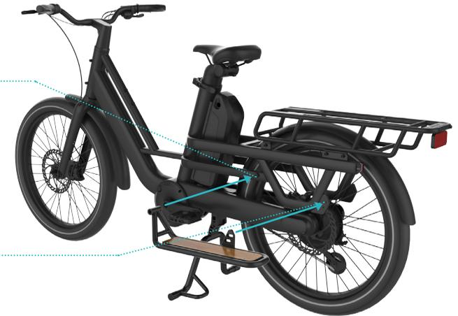
Align the right footrest with the screw holes of the frame, find the screws corresponding to the holes and tighten them.
