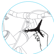
Target torque 12 \pm 0.5 \text{ Nm}
