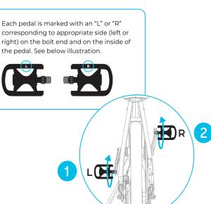
Target torque 30-35 N m
