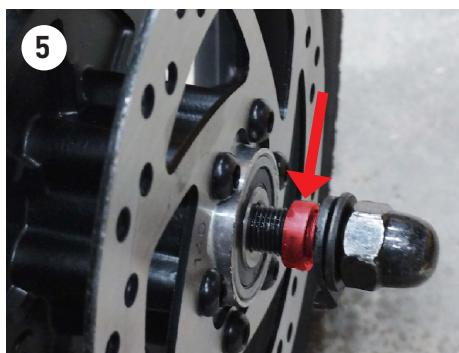
6. Fit the lock washers in the holes provided for that purpose, then tighten the wheel nuts.
