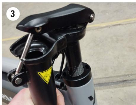
4. Raise the handlebar halfway, then tighten the screw in the centre.
