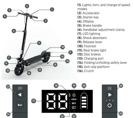
(17). Instant speed (18). Speed mode 1 (19). Speed modes 2 & 3 (20). Battery level indicator (21). Speed type indicator (22). Light activation indicator
